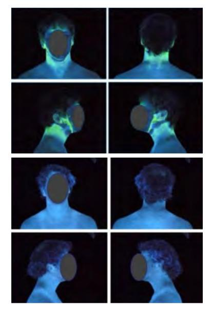
These results show the absence of particulates on the neck, shoulders and jawline of the test subject using the Smoke and Particulate Resistant Structural Turnout Ensemble prototype when used with one of the COTS particulate barrier hoods that are now available on the market (Responder News, 2016).
